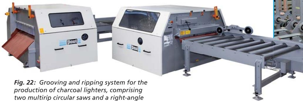
Fig. 22: Grooving and ripping system for the production of charcoal lighters, comprising two multirip circular saws and a right-angle transfer unit
