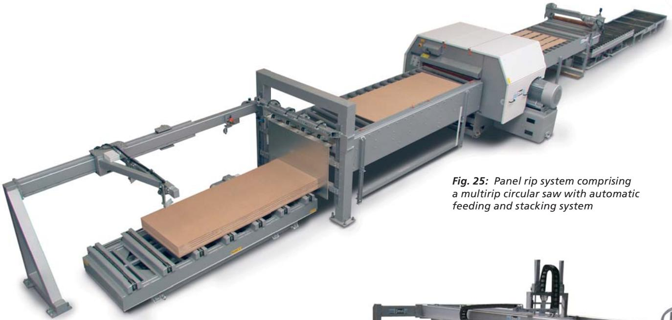
*Fig. 25: Panel rip system comprising a multirip circular saw with automatic feeding and stacking system*
