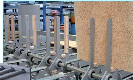
Fig. 23: Automatic panel turn-over device
